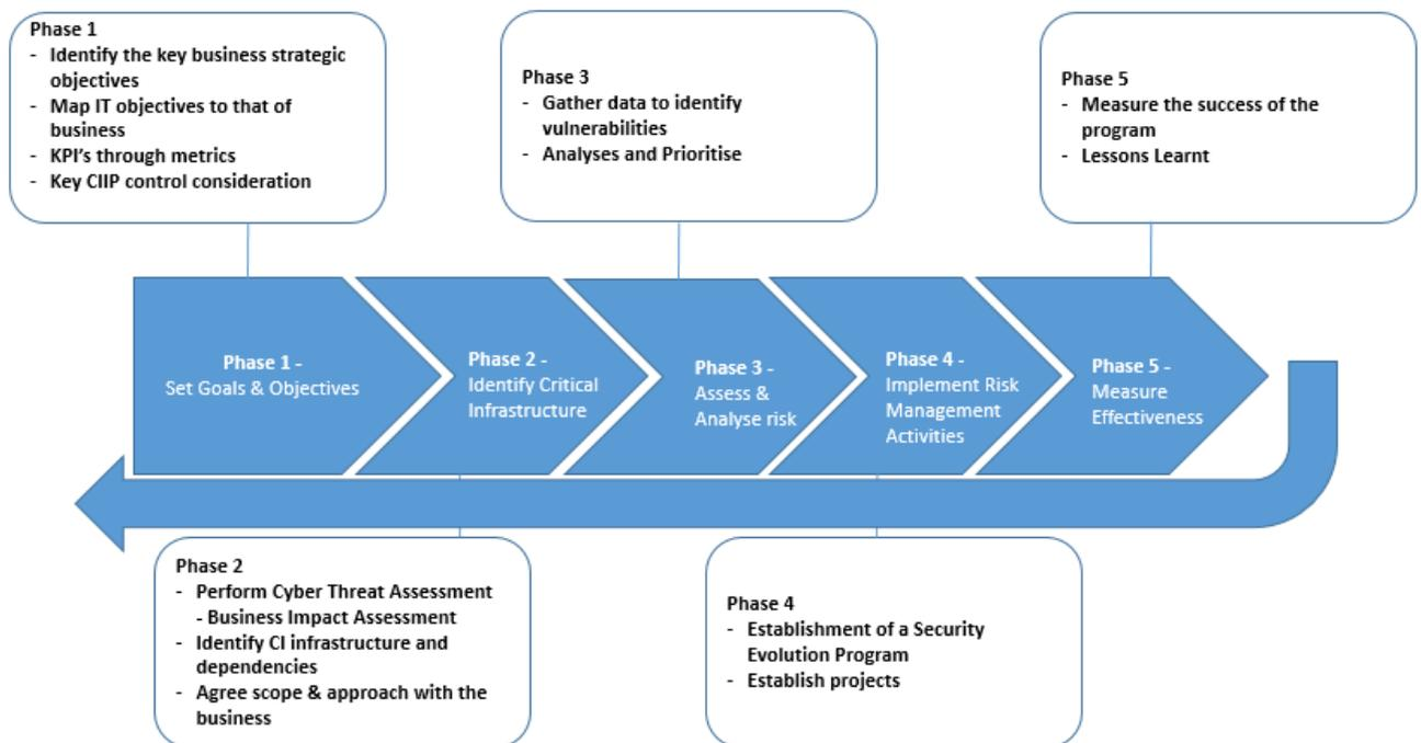
**Figure 3 - Proposed Hybrid Framework (After NIPP Framework)**
