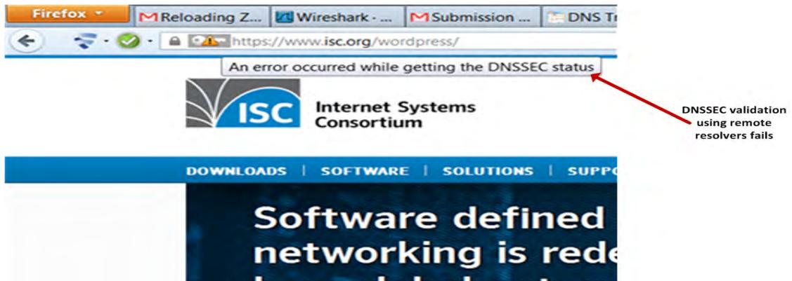
Figure 5.11: Remote Resolver Error Message
