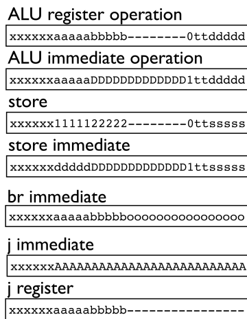
Figure A.3: Refined instruction encoding. Opcodes still take up 6 bits with the following changes in labelling compare with Figure A.2. ALU operations use two bits labeled with “tt” to represent the operand type (byte, short, word or long). A store.i instruction uses one register for the destination address labeled as “d” though it’s actually the register usually labeled as “a”, and a store instruction uses two registers for the destination address labeled with “1” and “2”. The source register for a store is encoded in the position usually used for a destination (labeled “s”)
