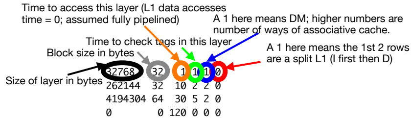
Figure B.1: Example of a configuration file. Each line represents a separate layer, unless you have a split L1 cache, in which case the first line is L1I (instruction) and the second line L1D (data). DRAM only has one parameter that is used, access time (misses from DRAM are not modelled – zeros are not permitted for sizes in other layers but are ignored in the DRAM layer).
