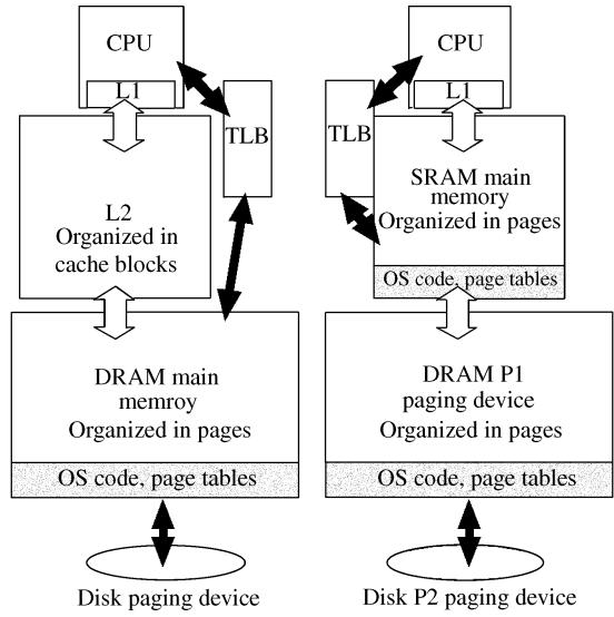
Fig.1. Conventional architecture (left) compared with RAMpage. (Major components are the same but organization differs. RAMpage uses the TLB to map the SRAM main memory instead of DRAM, and some OS code and data structures (shaded) are locked into the RAMpage SRAM main memory.)
