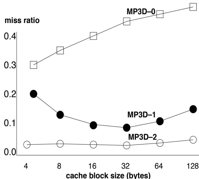
figure 1. Restructuring MP3D: memory simulation results
