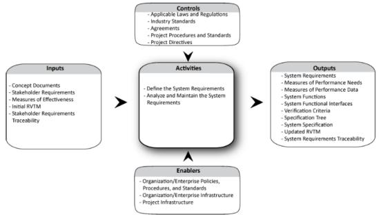
Figure 2-6: System Engineering Requirements Analysis Process (INCOSE, 2010)
