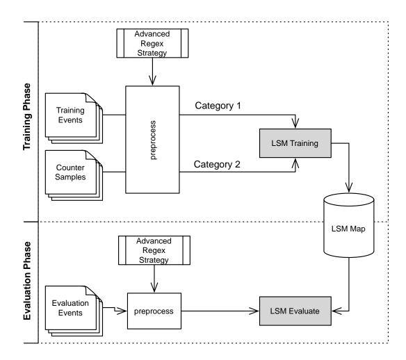
Figure 3.9: Use-Case 1 High Level Process Flowchart
