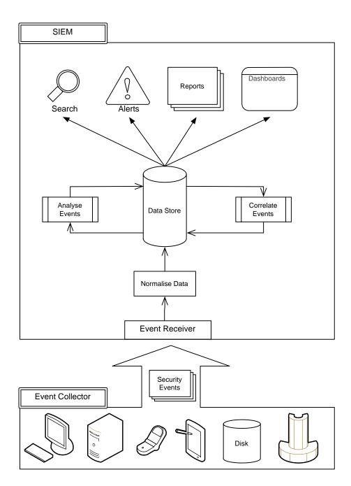
Figure 2.7: Diagram of a typical SIEM architecture
