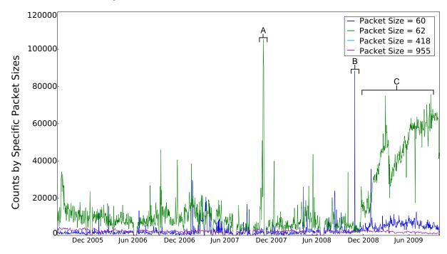
Figure 5.3: Packets Counts per Packet Size (/day).
