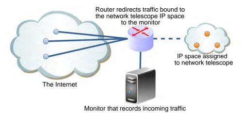
Figure 2.1: Components of a Network Telescope
