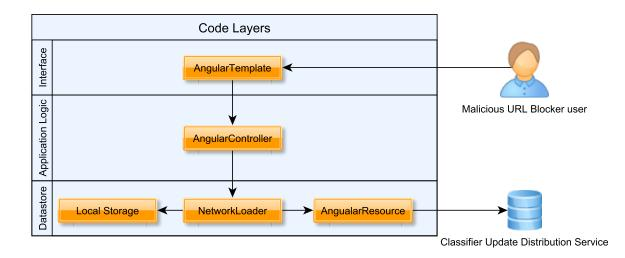
Figure 4.10: Layout of code structure within Net Defence.
