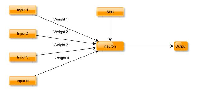
Figure 2.4: Basic layout of a perceptron.
