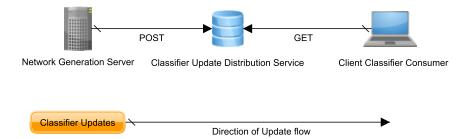
Figure 4.6: Flow of updates via Classifier Distribution Service (CDS).
