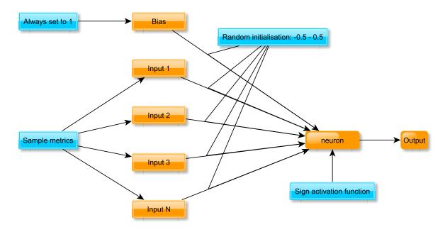
Figure 3.1: Structure and initialisation of the classifier.
